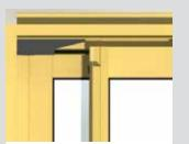
Series 461 windows are fitted with a tapered buffer stop to ensure the sash does not jump off the rail when opened.
