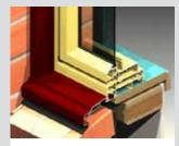
The detail above shows the ultimate frame finish with Longreach frame extender and the Paddington federation trims. The Paddington trims can be coloured to match, or contrast as shown above.
