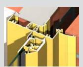
Standard 30mm jamb with built-in nailing fin/ weather bar into cavity brick wall illustrated above.
