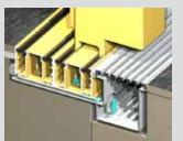
The sliding door detail shown above is ideal for high-end residential or commercial applications where you want a low flat sill that will keep water out.
