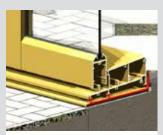
Sub-sill with central support leg designed to support the weight of heavy central door panels.
