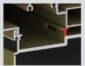
Stiffening rail in sill helps to support heavy panels and ensure smooth operation and long-term durability.
