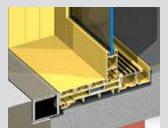
The above illustration shows the completely flat sill design. It features a four track XXXF flat sill with recessed sump on the outside and Centor™ SIE roller screen on the inside
