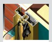
30mm jamb with built-in nailing fin/weather bar into brick veneer wall illustrated above.
