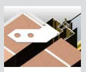
Alternative bold 44mm wide jamb with built-in nailing fin/weather bar. Both 30mm standard and 44mm wide nailing fin frames will accept height adjustable galvanised building-in lugs.
