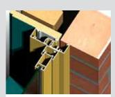
Standard 30mm jamb with built-in nailing fin/ weather bar into brick veneer wall illustrated above.
