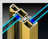
Sashes will accept glass from 4mm to 20mm thick. The ideal IGU is 16mm thick.
