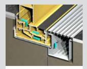
The sill can be recessed into floor finish and fitted with stainless steel drainage system.
