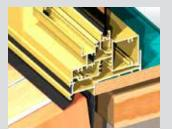
The nailing fin sub-sill shown above is standard on Series 452 windows. Ideal for brick veneer (shown above) or cavity brick wall construction.
