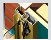
30mm jamb with built-in nailing fin/weather bar into brick veneer wall illustrated above.
