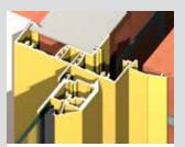
Standard 30mm jamb with built-in nailing fin/ weather bar into cavity brick wall illustrated above.
