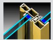
Series 462 sashes will accept glass up to 20mm thick. I6mm Insulated Glass Unit shown above.
