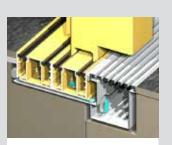
The sliding door detail shown above is ideal for high-end residential or commercial applications where you want a low flat sill that will keep water out.
