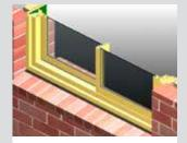
Double sash design with external sash fixed. Both fixed and opening sashes can be installed, replaced and/or reglazed from inside the building.
