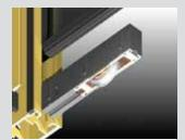
The key to making high performance sliding windows is to use large diameter, high performance wheels. We use sliding door wheels in the 602 and when the panels are double glazed or extra heavy, we use double bogey wheels.
